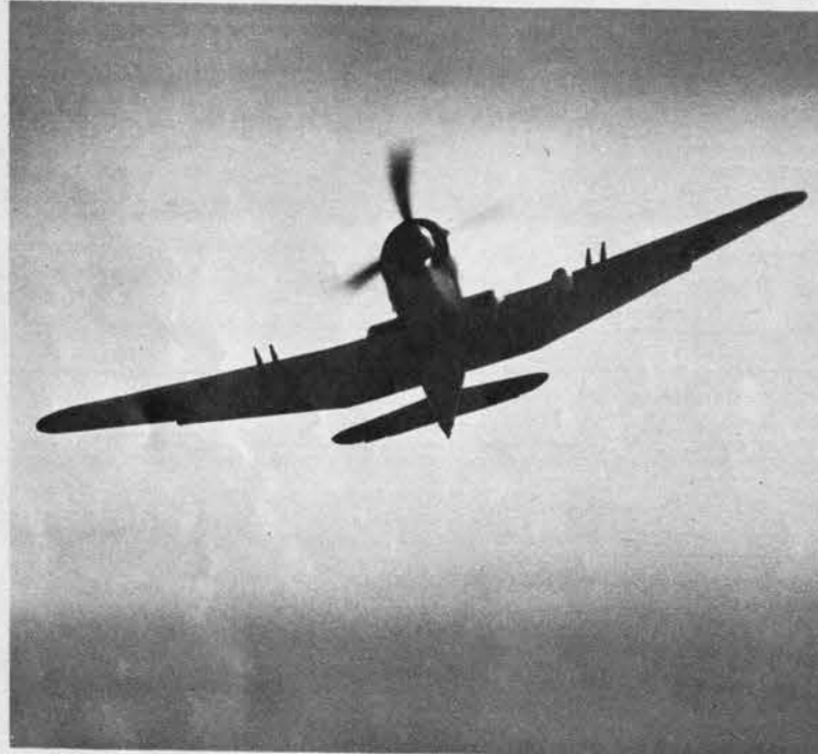
Firebrand's wing has straight inboard panel broken by two projecting air intakes. Training camera forms bump on the port outer panel.
